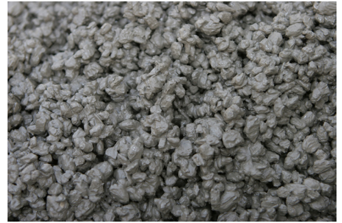
Pervious concrete fresh from the mix truck
